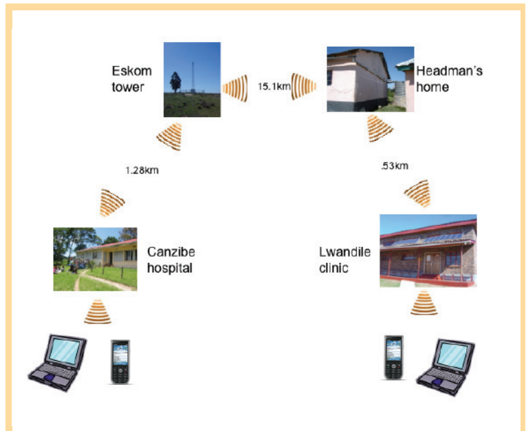
The hilly terrain and lack of line-of-sight between the hospital and clinic required two intermediate relays for the network. Each node costs about R4000, with a bit more for the solar sites. Either solar or mains charge a 12v 96aH battery. All network hardware was purchased locally in South Africa.
