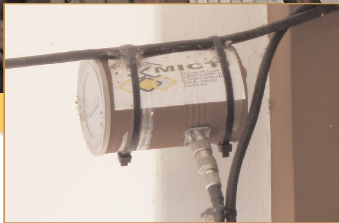
Low-cost can antenna (cantenna) made by MICTI students; installed and fully operational.
