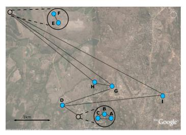
Fig. 2. A map of the Peebles valley mesh. Each solid dot represents a wireless node. An empty dot represents a close cluster of nodes shown in the circles. The area on the left is wealthy farm land and the area on the right is poorer tribal land.
