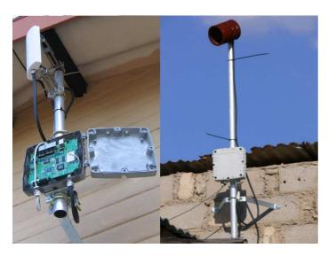
Fig. 3. Outdoor mesh node with repackaged Linksys WRT54G electronics in a waterproof aluminium case. The picture on the left shows an installation at node D is using a commercial 8dBi flat panel, the picture on the right shows an installation at node H which is using a home made Cantenna
