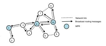
Fig. 1. OLSR routing protocol showing selection of MPRs
