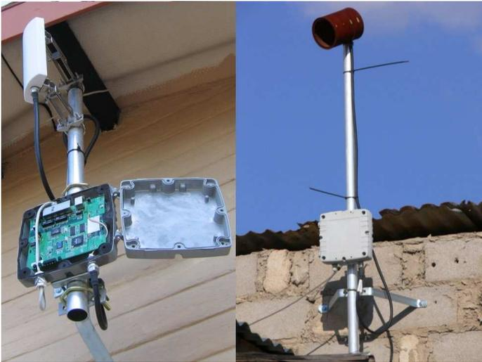
Fig. 3. Outdoor mesh node with repackaged Linksys WRT54G electronics in a waterproof aluminium case. The picture on the left shows an installation at node D is using a commercial 8dBi flat panel, the picture on the right shows an installation at node H which is using a home made Cantenna
